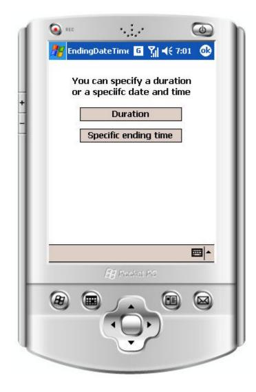
The ending date and time specifies the final time that the saved intervalometer program will run. You must always set an ending time and it must always be later than the starting time. You can choose an ending time up to several years in the future.
