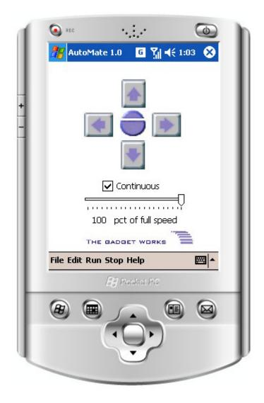
The opening screen appears when you start the program and when you return from any of the programming or editing pages. The opening screen contains <u>Directional</u> buttons that you use to manually move the robot right, left, up, and down. There are also buttons to fire the shutter and half-press the shutter release. To operate the controls you must be connected to the robot via Bluetooth.
